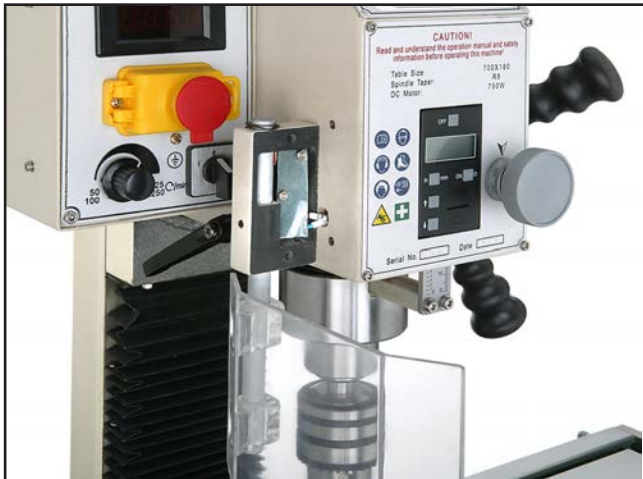
Figure 63. Chip guard limit switch.
